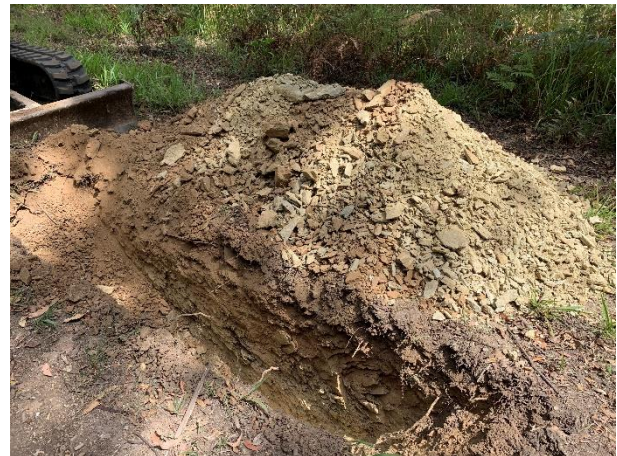
Highly to moderately weathered phyllite was encountered in TP6
